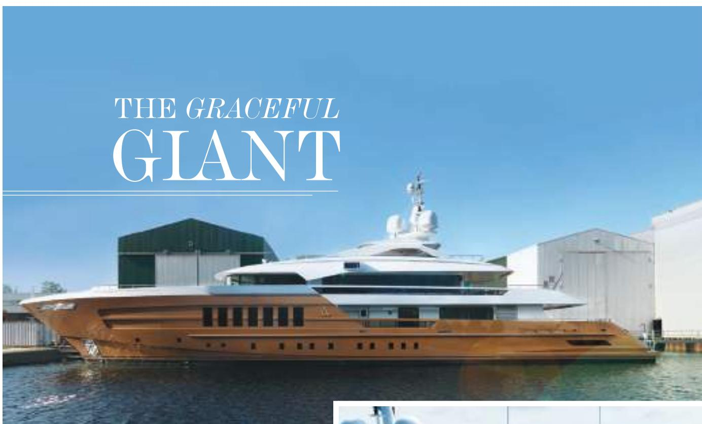
**S**ailing 180 feet of steel on some of the world's choppiest and coldest seas, while in unadulterated luxury, is no mean feat for the Azamanta. Made by Heesen Yachts, in partnership with Van Oossanen Naval Architects, this is the world's first fast-displacement yacht of its size made from steel. The patented fast-displacement hull form allows for greater efficiency of movement through the water at all rates of speed, not just those at the top.
